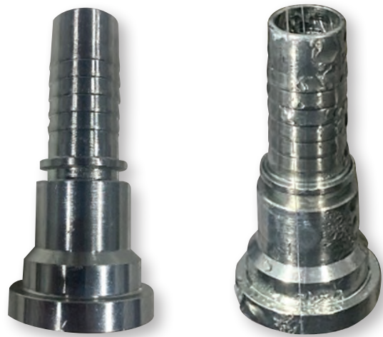
Left: Fitting prior to salt spray exposure. Right: Same fitting following 500 hours of continuous salt spray exposure.
